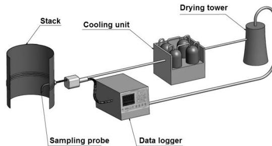
**Figure 2.** Scheme of gravimetric method
