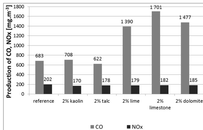
**Figure 3.** Concentrations of measured emissions CO and Nox
