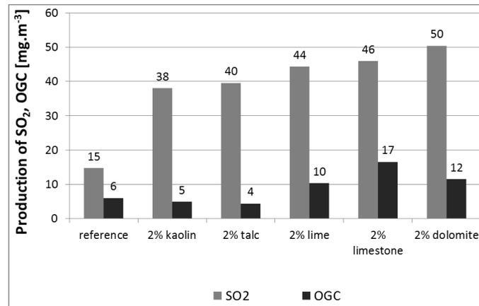
**Figure 4.** Concentrations of measured SO<sub>2</sub> and OGC
