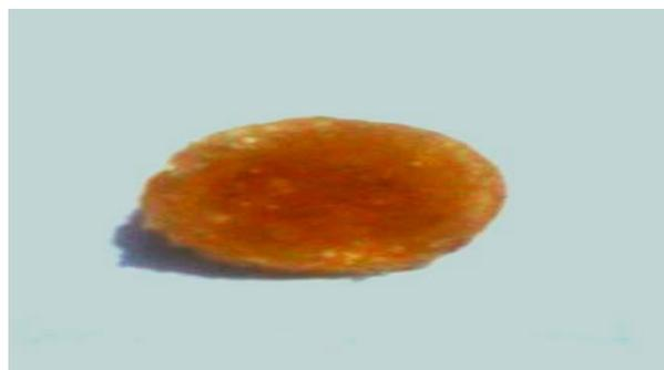
**Figure 2.** Synthesized Guar Gum-g-Poly (AAM) used as the adsorbent
