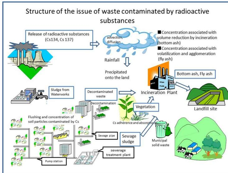
**Figure 3.** Pictorial diagram of radioactive contamination
