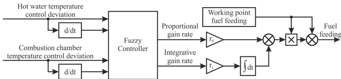
**Figure 3.** Block scheme of control algorithm using fuzzy controller
