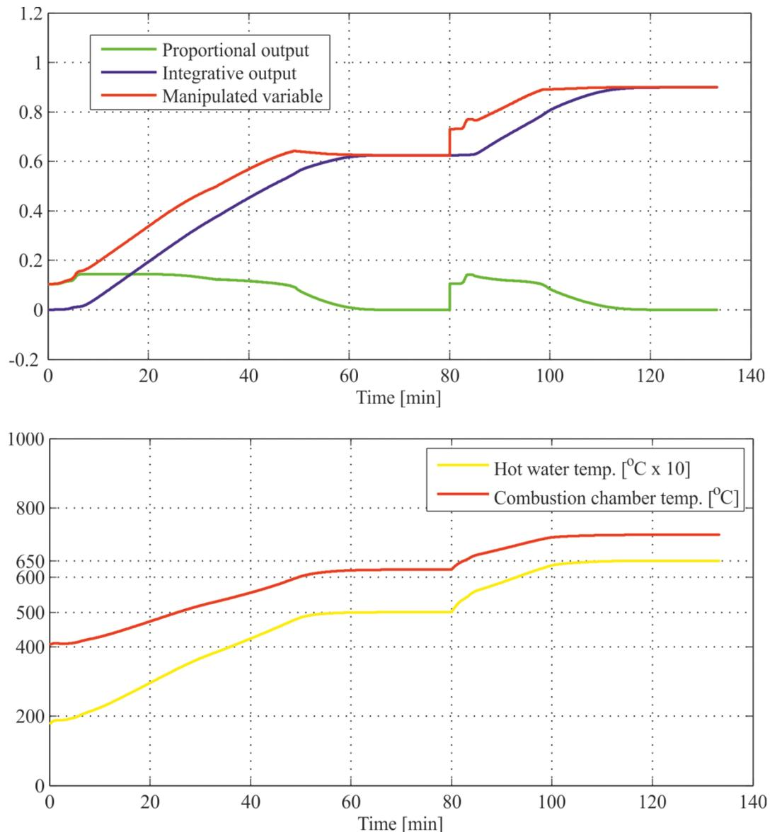
**Figure 4.** Simulation of set-point tracking control
