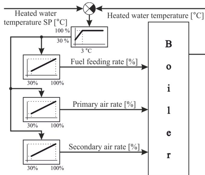
**Figure 1.** Scheme of a common method of small-scale
